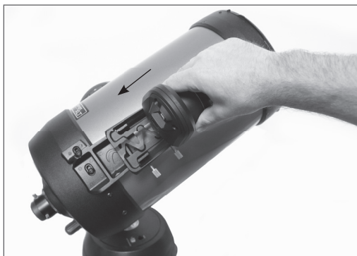
Installing large base (front to back)
